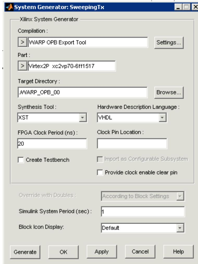
Figure 1: System Generator parameters for OPB core generation
